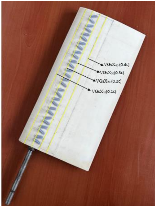
Figure 5: Location of XVGs on NACA 0012 airfoil
