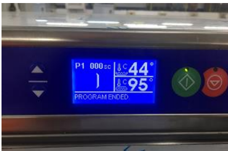
Figure 5: Temperature control screen of the innovative washer disinfector system prototype.
