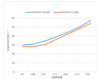
Figure 19. Channel output temperature graph according to amperage value
