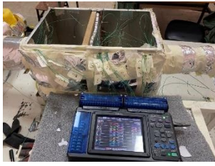
Figure 9. Visualization of the connection of thermocouples to the in-channel test setup with thermocouple connections of the data logger
