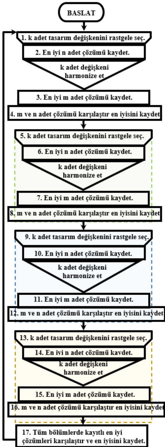
Figure 12. Artificial Harmonic Bee Colony Algorithm operation procedure.
