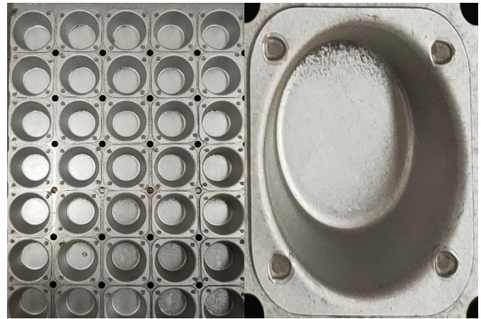
Figure 2: Welded Cake Pan and ROI Area
