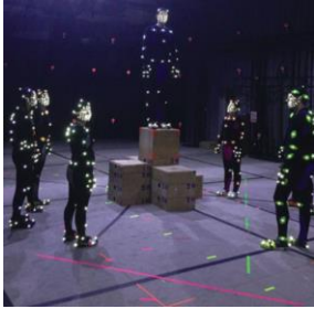
c) A marker-based outside-in optical tracking system. Multiple camera sensors are placed strategically in the environment, and the user wears several retroreflective markers to track the body and face.
