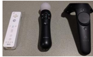
b) Examples of modern 3D mice that make use of optical and inertial sensing to produce 3D position, orientation, and motion data by mappings.
