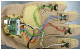
i) A multisensor data glove that uses accelerometers, gyroscopes, and magnetometers to capture information about each finger (active sensing).
