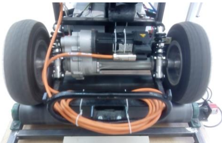
Figure 10: Propulsion of the disabled vehicle by using the PMSM.
