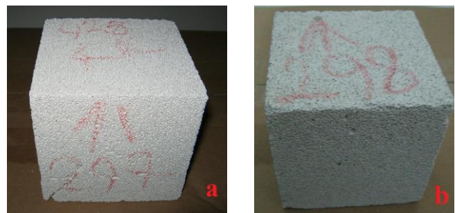
Figure 2. Macro images of the shaped aerated-concrete samples; a) F0 and b) F3
