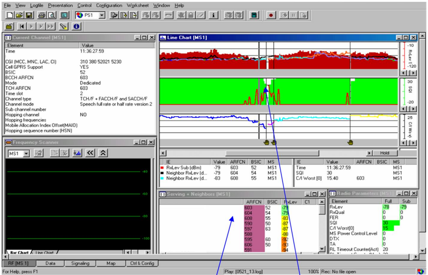
Frequency of serving cell is 603 and frequency of a neighbor cell is 604 Low C/I due to the co-adjacent interference
