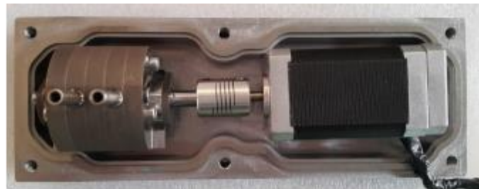
Figure 4.7. Compressor and motor placed in the semi-hermetic tank
