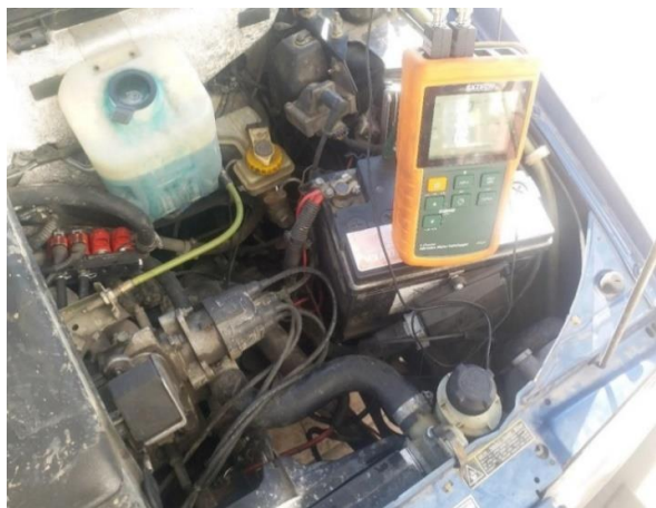
Figure 3: Engine Vibrations Measurement [3]
