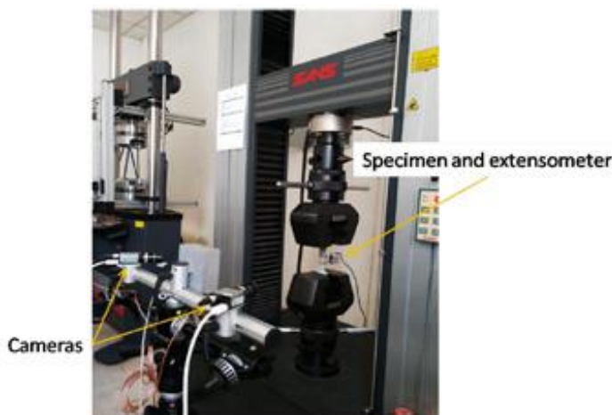
Figure 2: Test apparatus including digital cameras for direct tensile strength testing of titanium alloy plate [8].
