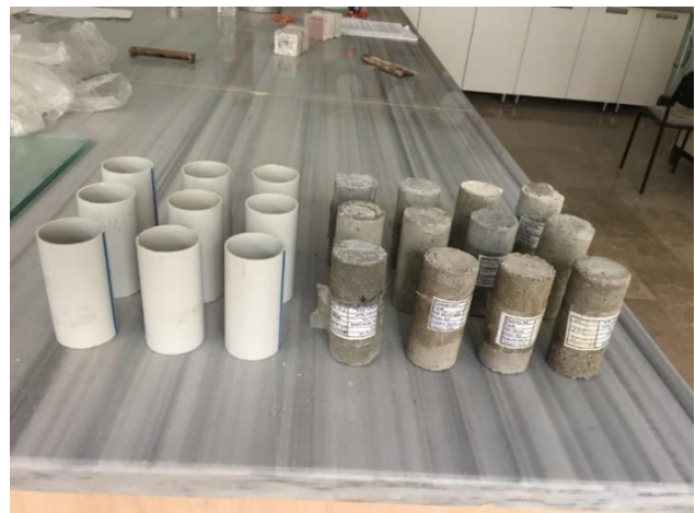
Figure 1: Cylinder specimens removed from the molds.
