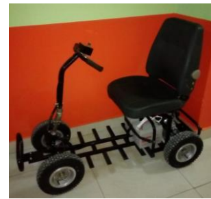
Figure 6: The electric mobility scooter to which PMSM will be mounted.
