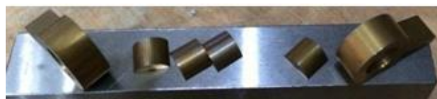
Figure 4.3. Piston and metal brushes coated with titanium
