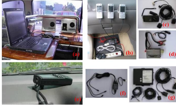
Figure 1: Drive test equipment (a) test tool (ready to measure) (b) TEMs phones (c) GPS (with external antenna and data cable) (d) 12V-220V inverter (e) GPS (vehicle mounted) (f) data cable and USB for phones (g) scanner (with external antenna GPS and RF, data cable)
