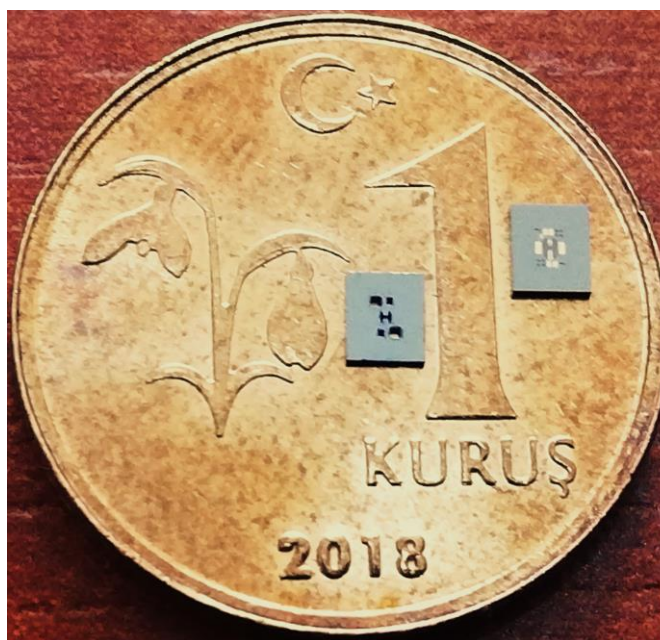
Figure 3: The fabricated shadow mask and a SOI based sensor in the die level.
