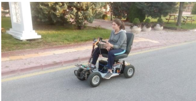
Figure 11: Testing the disabled vehicle which PMSM was mounted.
