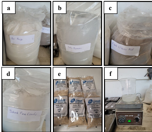
Figure 1: Binder materials (a) BA, (b) SD, (c) F-FA, (d) YFC, (e) CEN standard sand, and (f) alkaline activator.
