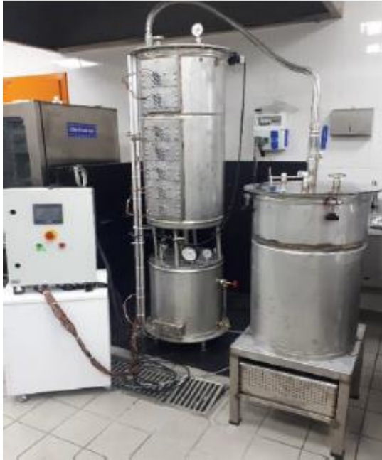
Figure 9: Photo of an innovative system prototype for steam peeling of various vegetable skins for commercial kitchens.
