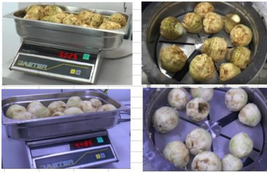
Figure 12 Photographs of celery peeling (before and after) on the innovative steam peeling system.
