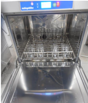
Figure 4: Photograph of the prototype of the innovative washer disinfector system that provides effective drying and cleaning (basket with a glass beaker).
