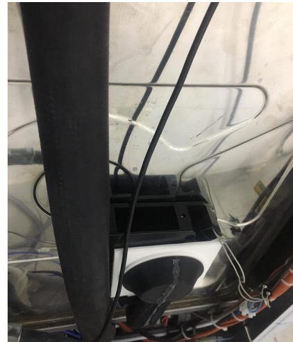
Figure 7: A photo of the fan drying system (on the back side) of the innovative washer disinfector prototype.
