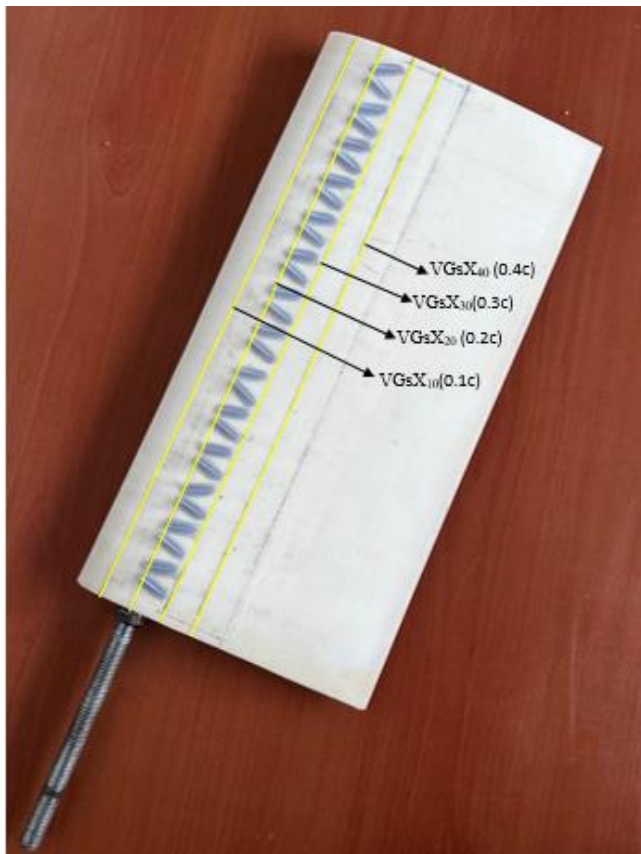
Figure 5: Location of XVGs on NACA 0012 airfoil
