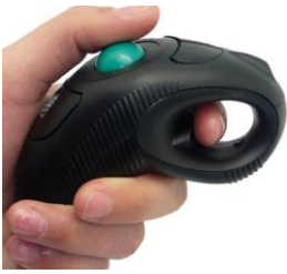
a) a handheld wireless trackball device used in AR, mobile, and immersive 3D environments.
