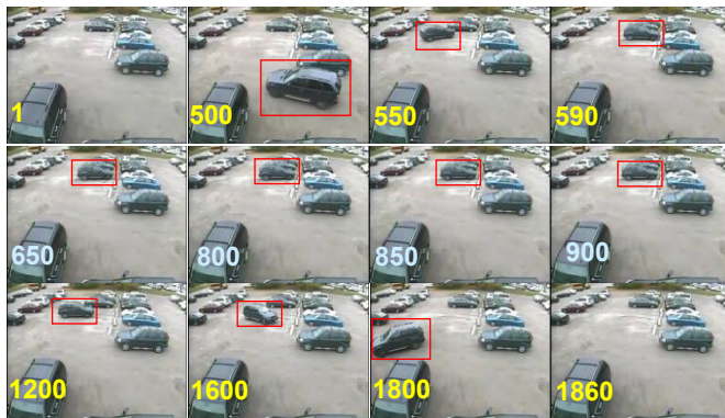
Figure 2: The blue written frames fake frames were pasted over the frames in Figure 1 to cover the moment of the accident with duplication forgery
