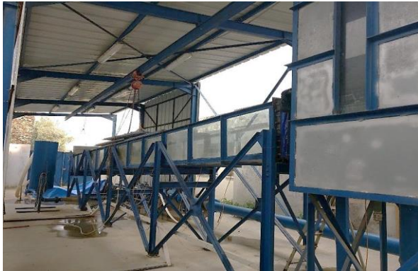
Figure 3: Experimental Setup at the INAT laboratory (Length: 10m; width: 0.8m; Height: 0.6m)
