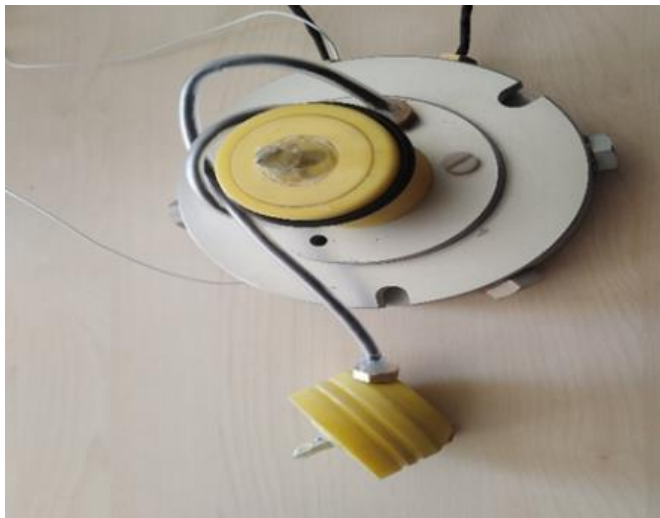
Figure 2: Triaxial test top and bottom cap with bender elements.
