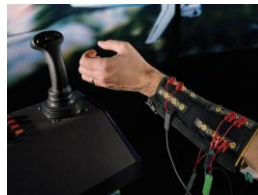
j) An example of a device that tracks finger movements and gestures by using EMG sensors to detect muscle activity in the forearm (active sensing).
