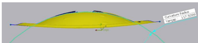
Figure 4. Measurement of curvature radius of bulged sheet
