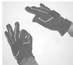
h) A conductive cloth-based Pinch Glove (conductive cloth at each of the fingertips, active sensing).
