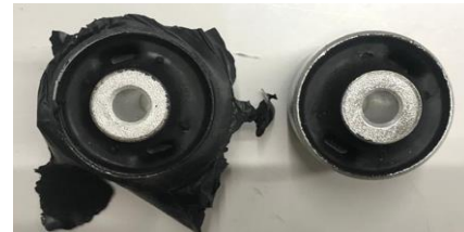
Figure 1: Uncleaned and cleaned sample bushing.
