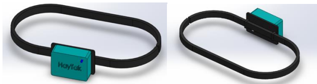
Figure 2: Visual of the designed neck collar – front face (left) and back face (right).
