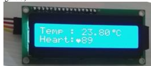
Figure 5: The display of body temperature and heart rate with biosensor system
