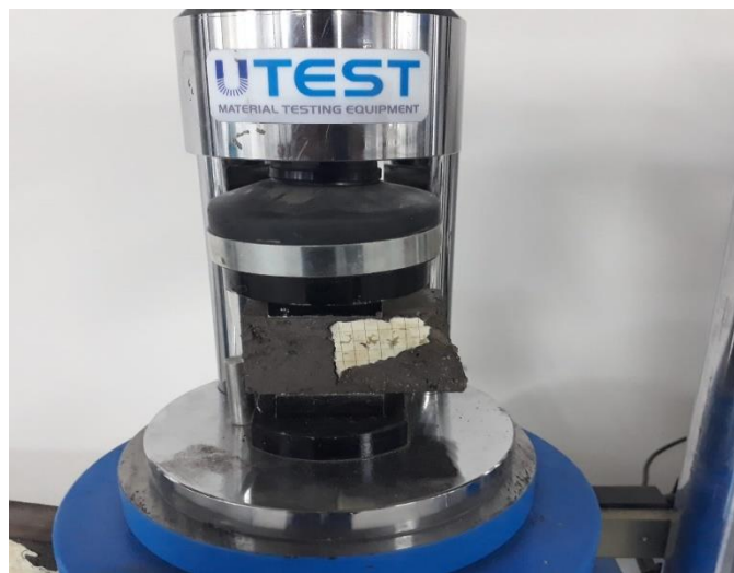
Figure 1. Compressive strength test of geopolymer mortar
