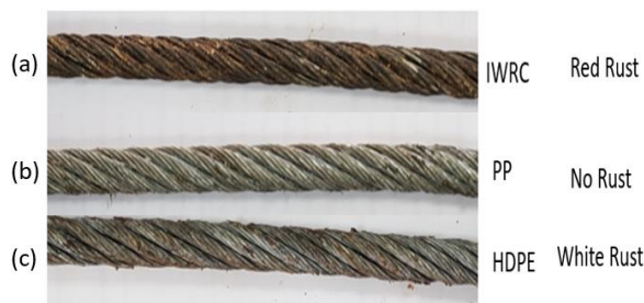
Figure 6. Rust condition of steel core (a) IWRC, (b) PP, (c) HDPE
