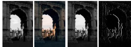
(e) Bilateral Filter (f) Guided Filter (g) Anisotropic Diffusion Filter (h) Sobel-x Filter
