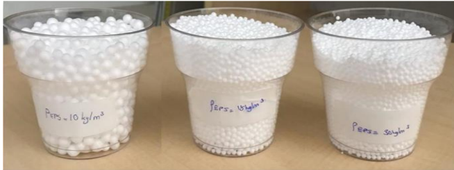
Figure 1: EPS beads with the density of 10 kg/m 3 , 18 kg/m 3 , 30 kg/m 3 , respectively.
