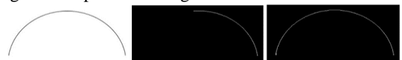
Figure 6: From left to right: open counter curve to be traced, the result of clockwise tracing and result of both clockwise and counter clockwise tracing.
