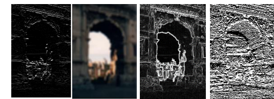
(i) Sobel-y Filter (j) With \sigma = 10 Gauss Filter (k) Gmag Filter (l) Gdir Filter
