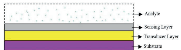
Fig. 1 MEMS-based gas sensors layer structure
