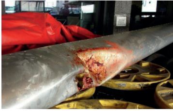
Figure 2: Bird strike damage to B737 aircraft left wing leading edge [3].
