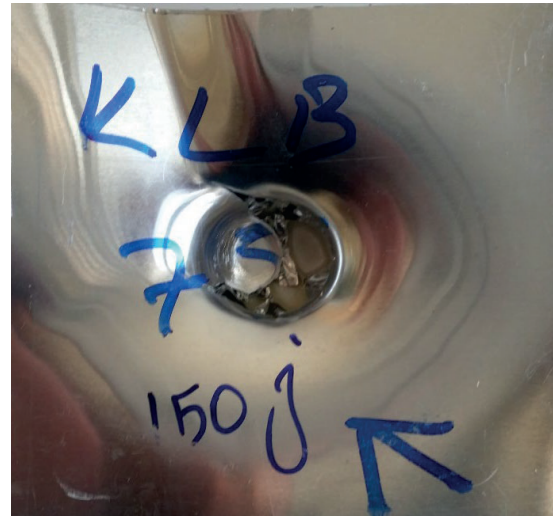
Figure 5: Front image of sandwich panel impacted at 150 J energy level.
