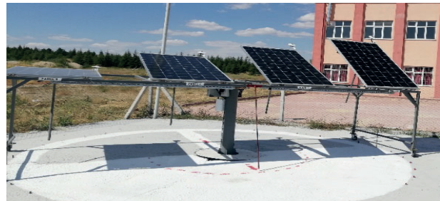
Figure 2: Movable PV panel to set tilt and azimuth angle
