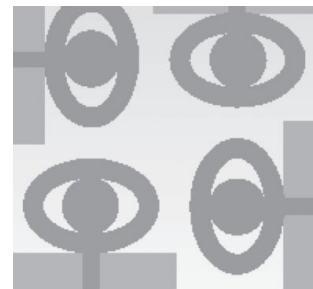
Figure 7: 4 \times 4 MIMO antenna structure.
