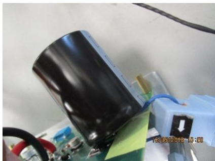
Figure 9: Measurement connection of dc bus capacitor current
