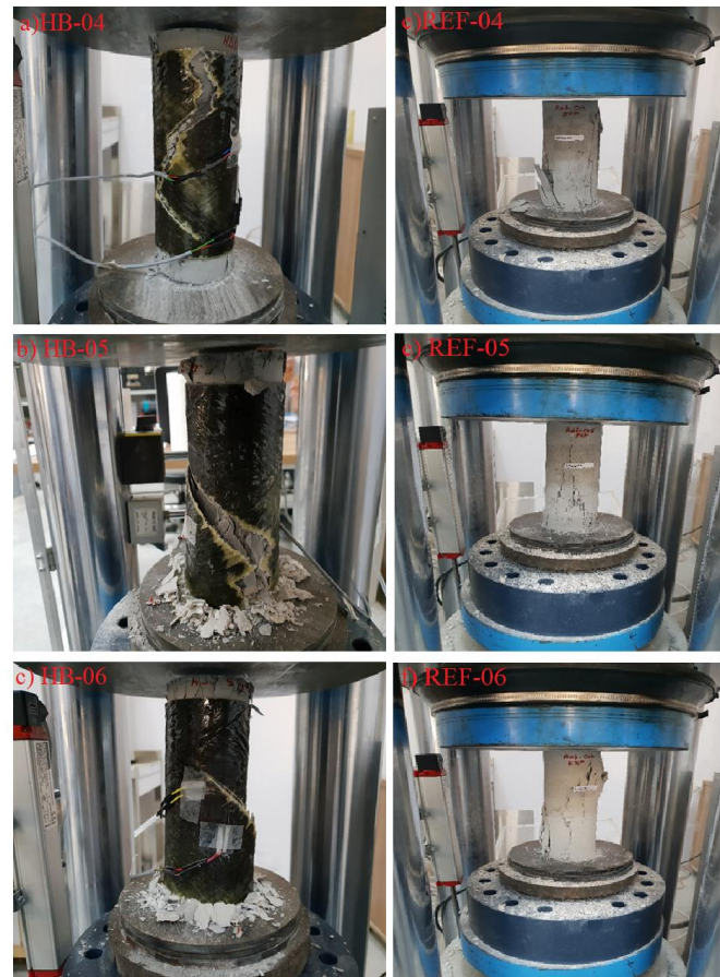
Figure 2: Fracture damage of specimens after testing
