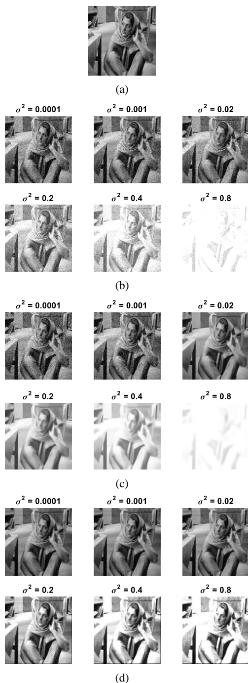
Figure 2: (a) The original image “Barbara”, (b) Degraded image with different AWGN noises (c) BM3D algorithm denoising results (d) 2D ZA-LMS algorithm denoising results
