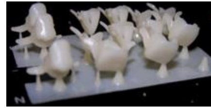
Fig. 17. Applied of Arch models built in plaster like material on 3D Printing system [10]
