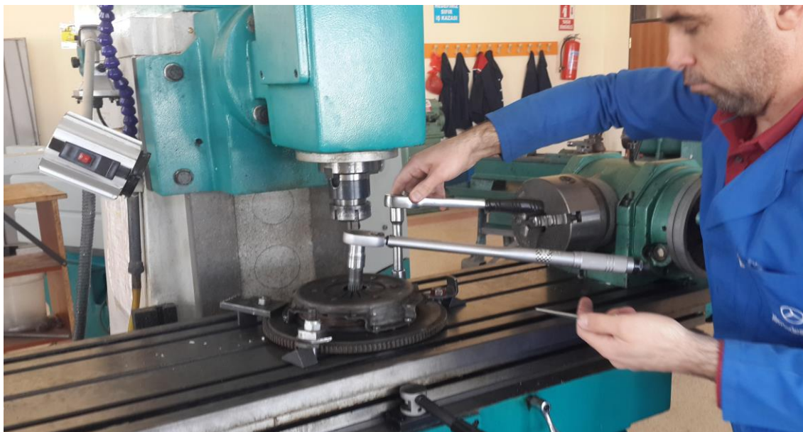
Figure 4: Torque measurements of the dry clutch fixed to the experimental system
