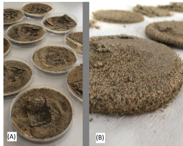
Figure 3. Results of sand hardenin (A: Without inoculum; B: With inoculum)
