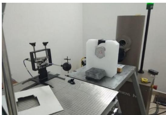
Figure 3: Cs-137 gamma irradiation system and geometry.
